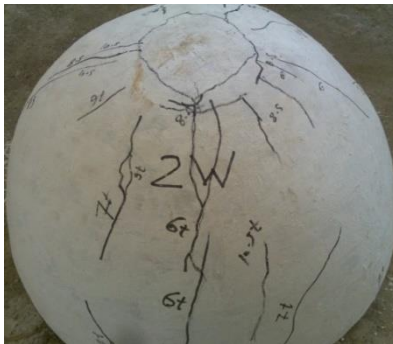
Fig. 6-A : Cracking patterns for all tested domes D1
